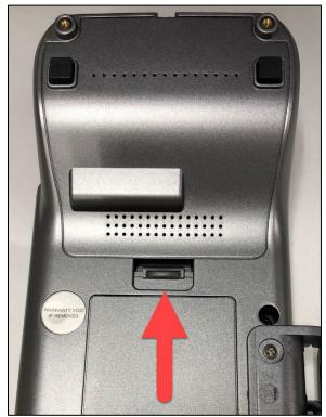
3. Insert the data cable into the HDMI connector and route the cable through the recesses provided.
