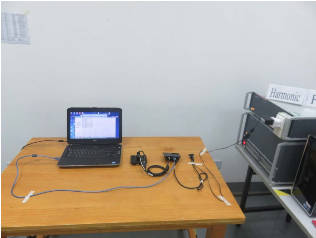
Picture 4 Harmonic Current Emission & Voltage fluctuation and flicker Test Setup
