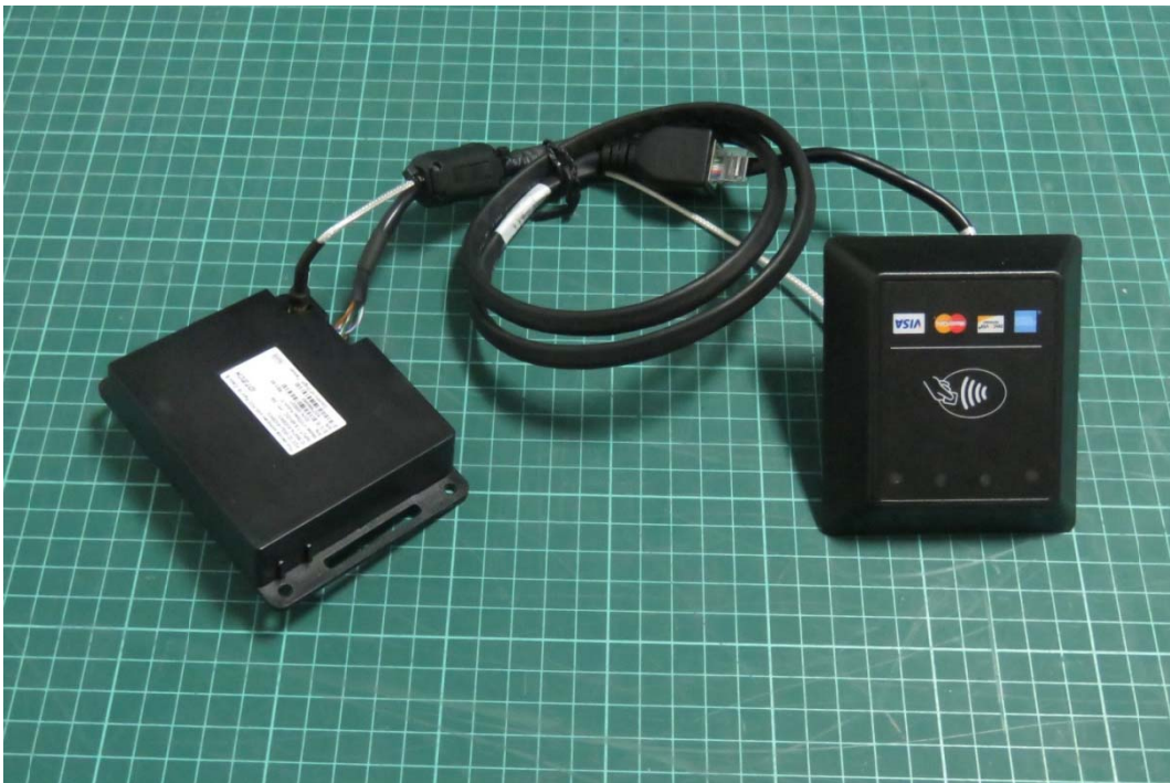
controller D & Antenna C ViVOpay Kiosk III SRED Picture 1 Constituents of EUT
