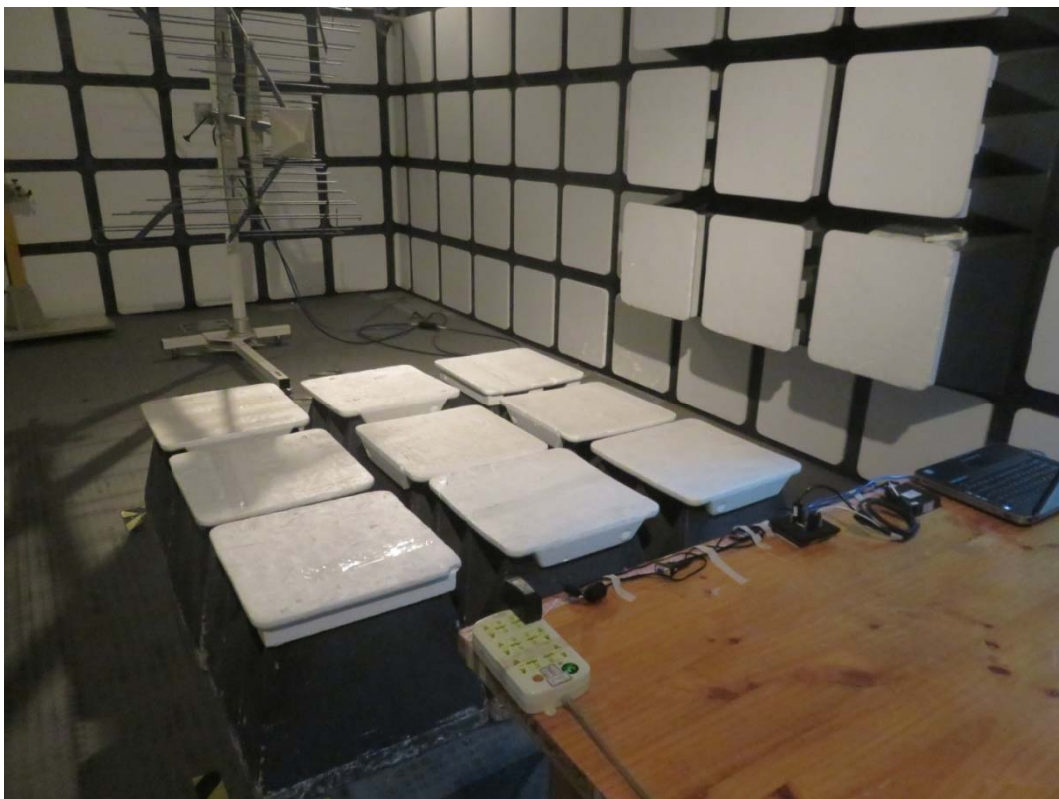
Picture 7 RF Electromagnetic Field (RS) Test Setup
