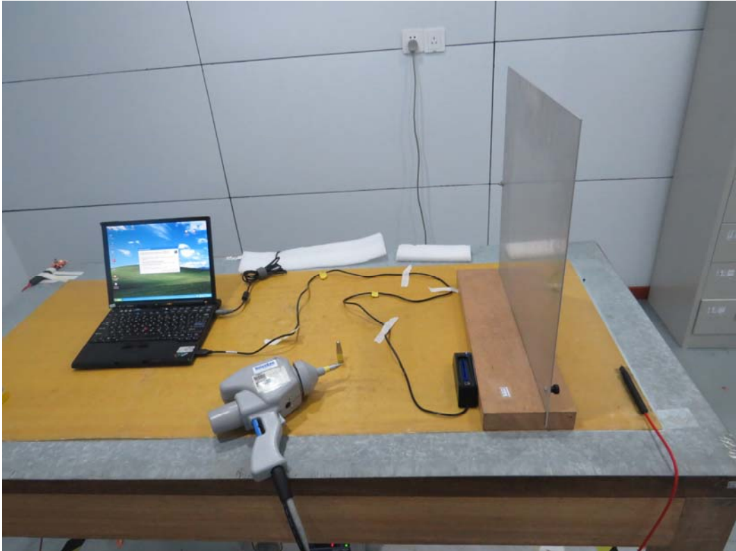
Picture 2 Electrostatic Discharge Test Setup
