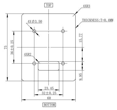
**Note:** Verify the orientation of the Kiosk V before marking and drilling the holes. The **rectangle** hole should be located towards the bottom of the mounting location to ensure that the Kiosk V is oriented correctly with the LEDs at the top.
