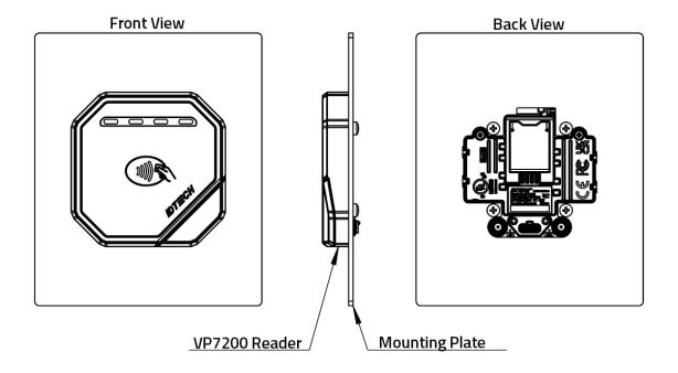
**Note:** The VP7200 is post-compatible with Kiosk III, Kiosk IV, and VP7200 dimensions. Posts are 36mm apart in the lengthwise direction and 32mm apart widthwise. See the drawing below.
