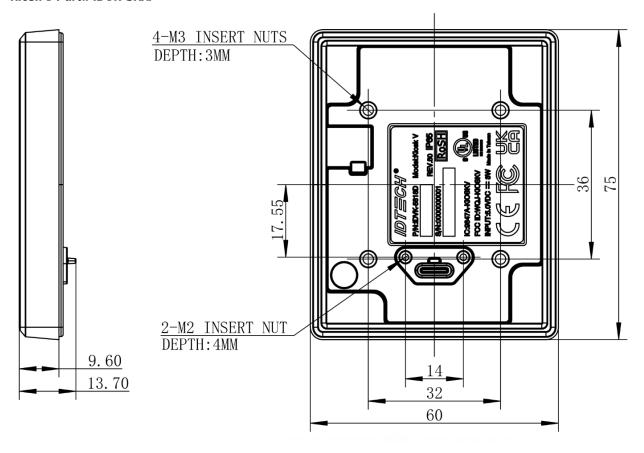
**Note:** The Kiosk V is post-compatible with Kiosk III and Kiosk IV dimensions. Posts are 36mm apart in the lengthwise direction and 32mm apart widthwise. See drawing below.
