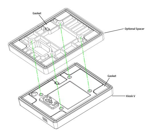
2. Place the second gasket module on the optional spacer; if the gasket and spacer have separated, assemble the gasket to the spacer according to the diagram below.
