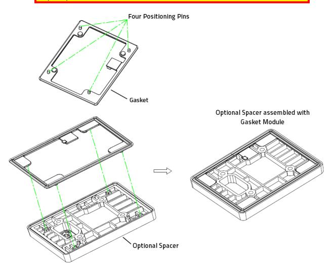
3. Insert and tighten the four M3 screws to mount the spacer assembly to the metal backing plate.
