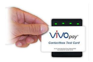
The Kiosk V should beep, and the four green LEDs should illuminate in sequence, then all will illuminate together, briefly (750 msec), to indicate a successful test.
