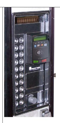
Connect the power cable into the electrical outlet. The ViVOpay Vendi unit LEDs should come on and the unit should beep.
