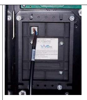
Attach the other end of the Pigtail Cable to the supplied Interior Cable, which then attaches inside the vending machine. Tidy all cables and fasten with nylon cable-ties. Ensure that no loose cables could be caught when the vending machine door is opened/closed for servicing. Additionally, avoid routing excess cables over fans or other electrical motors that could cause undue heat buildup or electrical interference.
